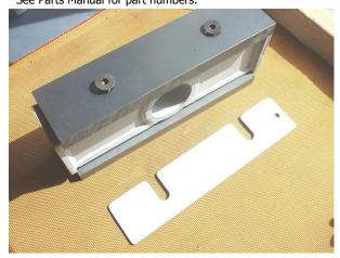
20 CHECK THE CONDITION OF THE BODY TO CHASSIS MOUNTING PLATES, BRACKETS, HARDWARE , AND SPRINGS...MONTHLY
